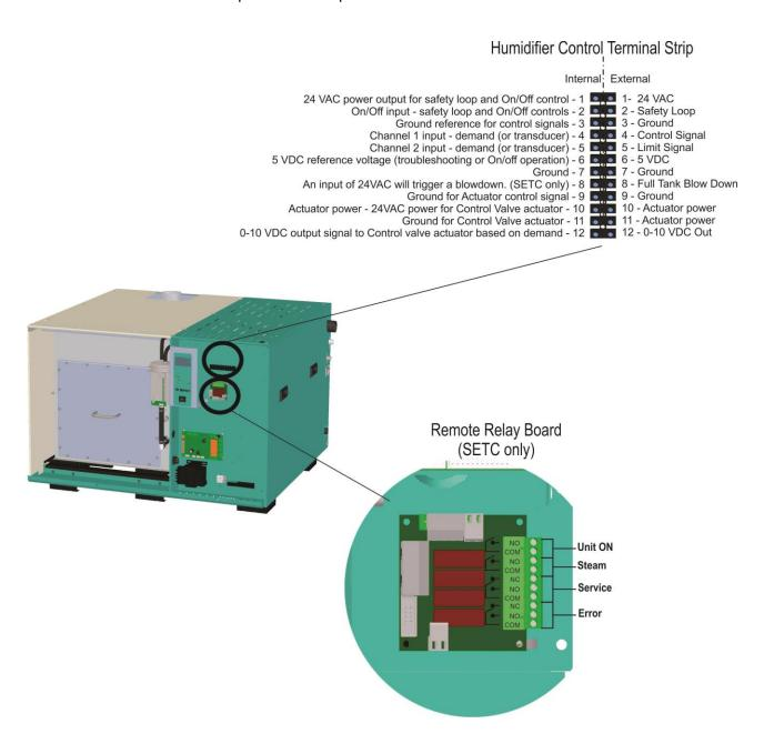
Figure 29: SE Humidifier Control Terminal Strip
