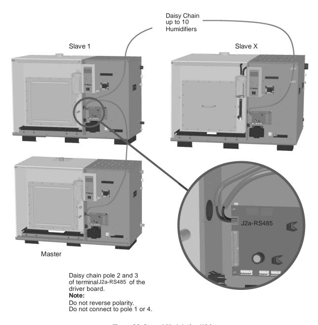
Figure 30: Staged Modulation Wiring
