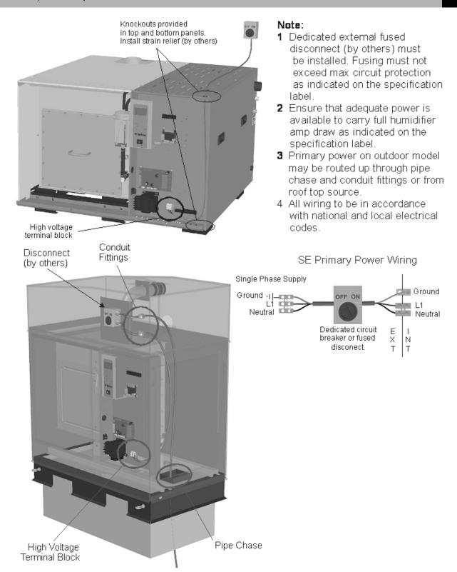
**Figure 21: Primary Power Connections**
