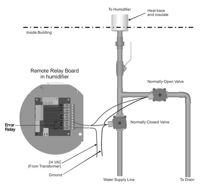
Figure 18: Freeze Protecting Water Supply
