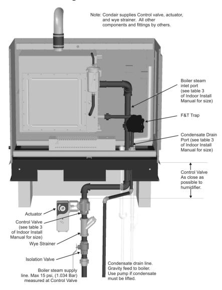
Figure 20: SE Outdoor Boiler Steam and Condensate Connection
