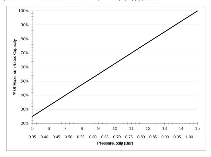
Figure 10: Output as a Function of Supply Steam Pressure
