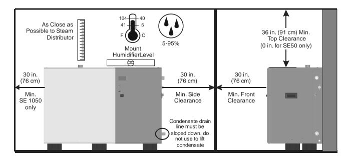
Figure 11: SE Indoor Installation Location / Clearance
