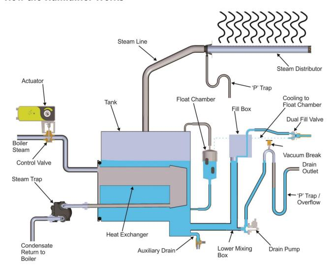
Figure 1: Humidifier Schematic
