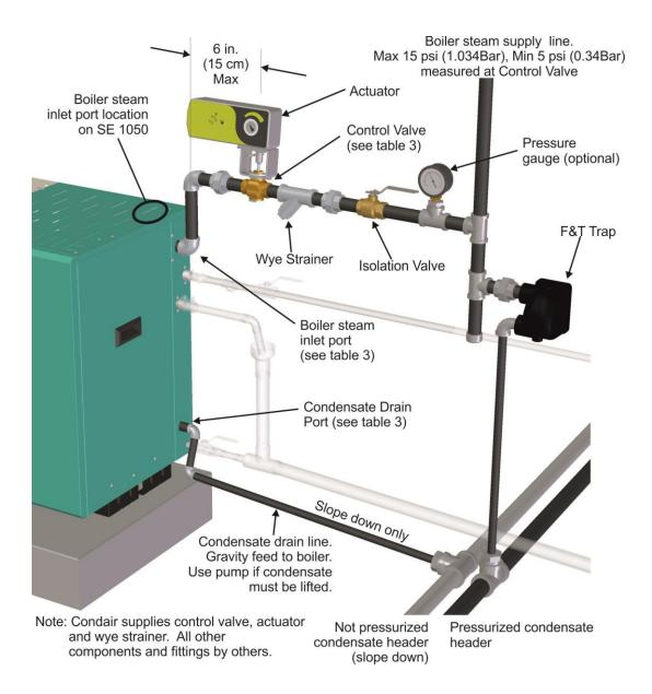
Figure 19: SE Indoor Boiler Steam and Condensate Connection
