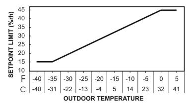
Figure 27: Outdoor Temperature Reset
