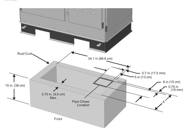
Figure 15: SETC Outdoor Roof Curb
