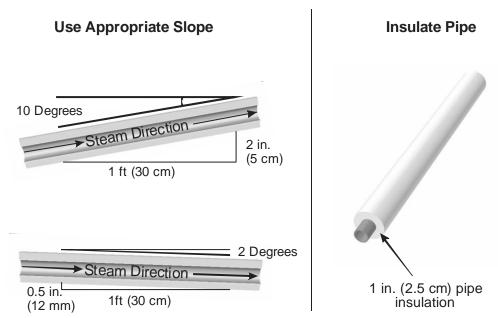
Figure 23: Main Steam Line Requirements
