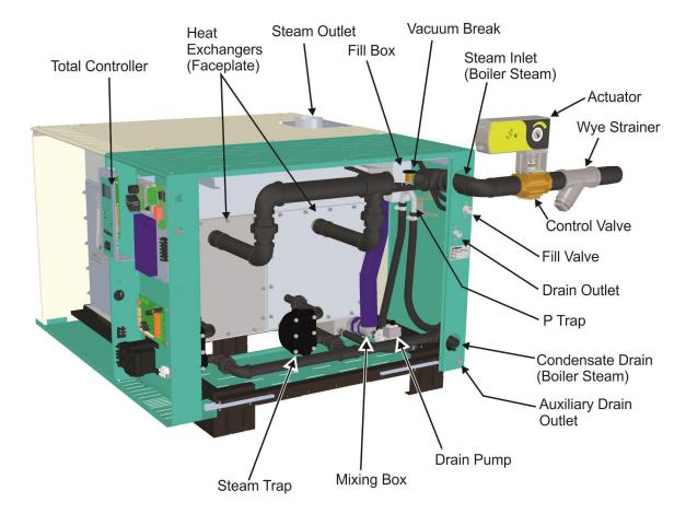
**Figure 5: SETC Humidifier Components**
