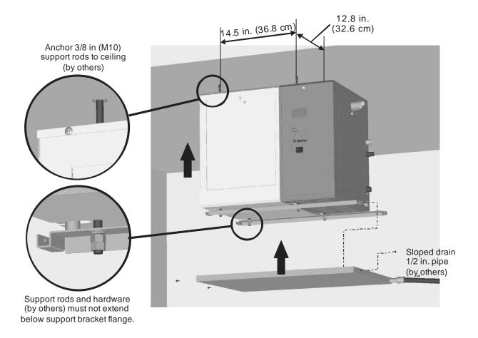
Figure 13: Ceiling Mounting the SE50
