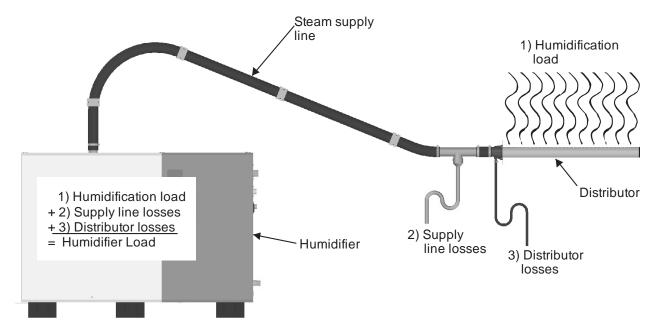
Figure 9: Humidifier Load
