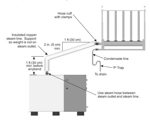
Figure 25: Steam Distributor Above Humidifier (Copper Steam Line)
