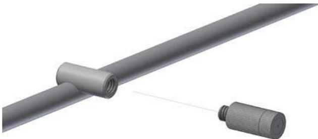
Fig. 20: Insertion des buses
