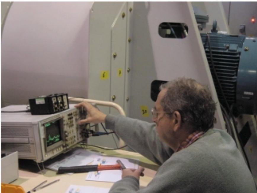
A laboratory with a full complement of measurement equipment: over-speed installation, fatigue tests, test rigs for measuring fan performance, noise and vibrations, according to the latest international standards.
